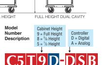
For Standard Wattage Cabinets (120V, 12A, 60Hz, 1400W)
