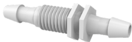
BH1428-2-2-200 Bulkhead Adapter • 1/4 inch – 28 UNF Thread • 1/8 x 1/8 inch Barb
