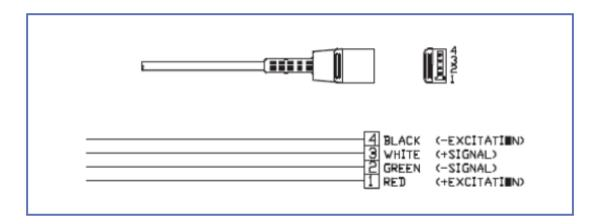
Reusable Cable which connects to the monitor/control system has five wires-four as shown above and the 5th which is a cable shield (silver)
