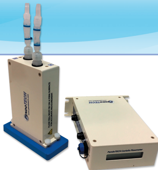
Complete flowmeter shown (model PCFM-32)
