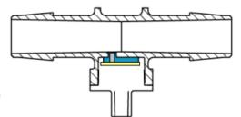
Figure 1. Illustration of pressure sensor body with chip inserted Yellow: ceramic base of the chip which contains all electronics Blue: Chip housing which bonds to sensor body Gray: Dielectric silicone in chip housing that isolates fluid path from electronics and conveys pressure
