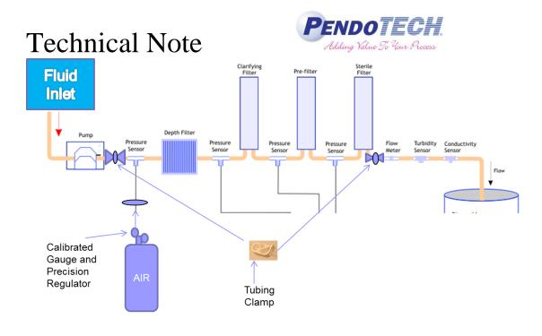
Figure 5. Illustration (for representation only) of a test set up where a calibrated reference pressure could be compared to pressure sensor readings.
