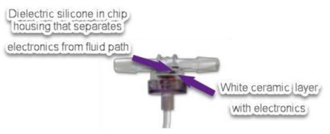
Figure 2. Photo of pressure sensor body with chip inserted
