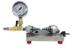
A precision regulator connected to an air source and calibrated gauge (calibrated gauge and precision regulator not shown) can be connected to inlet connection on the left side shown below. With the isolation valve open, the calibrated gauge reading can be
