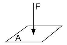
This force can be then normalized to force per unit area such as pounds<sub>force</sub> per square inch (psi) or in SI units as Newtons/m<sup>2</sup> or Pascal (Pa) or expressed as other relative measurements such as mm of Mercury (mmHg), Bar, or Atmospheres (atm). Standard atmospheric pressure (1atm) is defined as 1.013bar, 101.3 kPa, 760mmHg, and 14.7psi.
