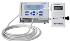
This has an upper test limit of 10 psi which is the PressureChecker limit because it is designed for high resolution readings and the limit of the calibrated internal reference pressure transducer (that reads on the LCD).
