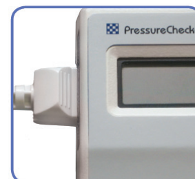
Sensor simulator port for testing monitors only
