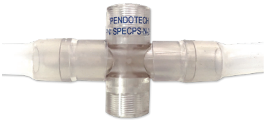
1cm flow cell with tubing installed
